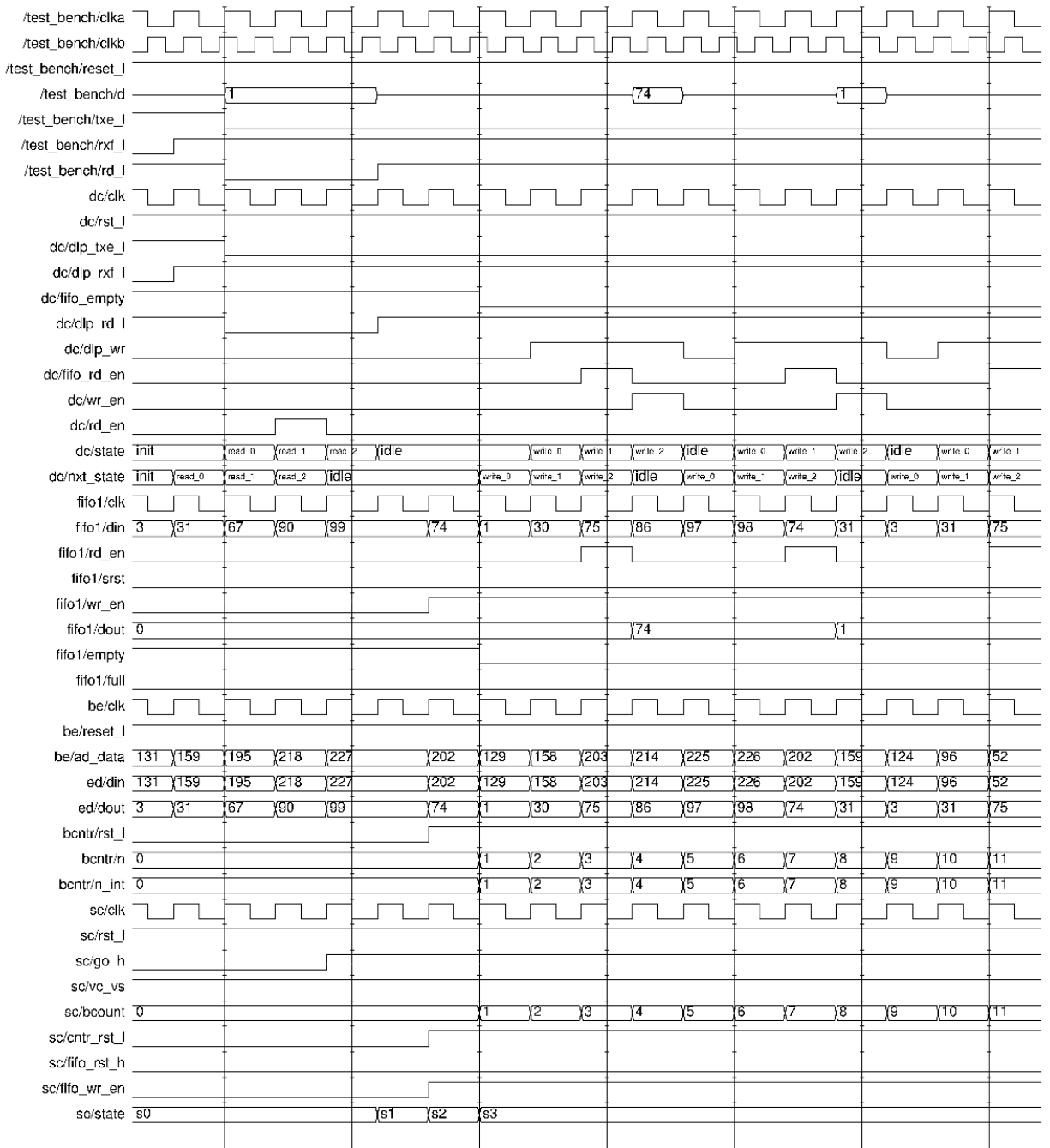
Fig. 29. Timing diagram verifying the operation of the DC100 within its test architecture: 1 is read from the DLP, and 74, 1 read from the FIFO and written to the DLP.
